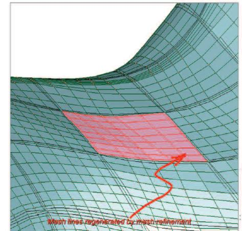
Mesh lines regenerated by mesh refinement
