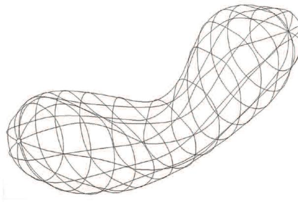
Input: polylines are imported as a .dxf into Robot
