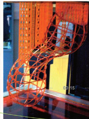
**1** In the SLA technique the system creates a platform from which the 3D model must be oriented and positioned. The physical part is built on a base platform of a glass plate. This corresponds to the digital representation in the software and is referred to as the build bed.
