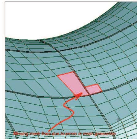
Missing mesh lines due to errors in mesh generation
